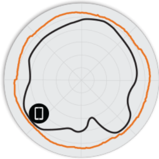
Figure 2. T310d 2.4GHz Azimuth Antenna Patterns
